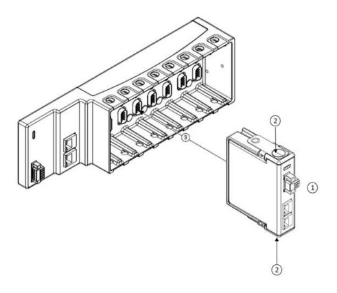
Complete the following steps to install the cRIO ECAT module in a cRIO chassis.
